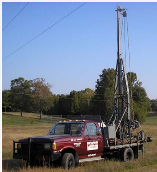
BCD's Mobile B-31 drill rig (Memphis Office)
